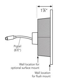
iSteam controls flush mount in the steam/shower enclosure through a 5-1/4" wide x 3-9/16" high hole. iSteam controls can also be surface mounted. They are suitable for use with SteamLinx $^{\text{m}}$  mobile app control.
