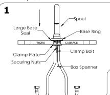
• Assemble the spout by placing the hoses through the Ø1. 3/8" hole in the work surface, ensuring the base ring & rubber seal
