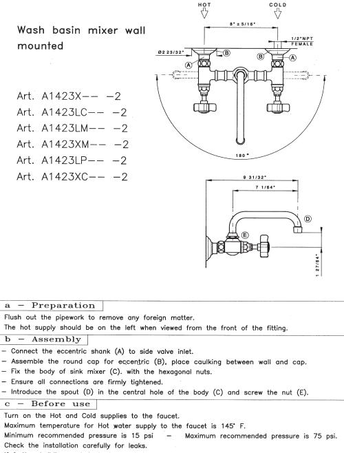
If further building work is to be carried out in the vici of the faucet, it should be covered to prevent paint, adhesive, etc. from damaging the surface.
