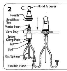
Sidevalve to be installed from underside of work surface as shown.
